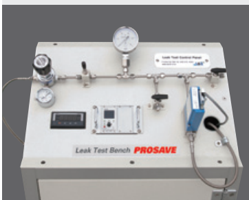
Test bench of opening pressure / vacuum and seat leak test of P/V valves
